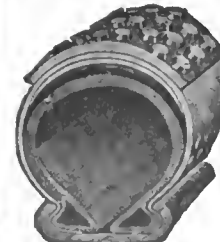
Sectional View of Casing MADE NEW. Note the hardened steel anti-skid studs at the top, the split needle rivets just above the rim and the strip of canvas inside to protect inner tube
